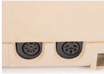
» The AV Jack is on the left, while the serial port on the right handles devices such as printers and disk drives.
